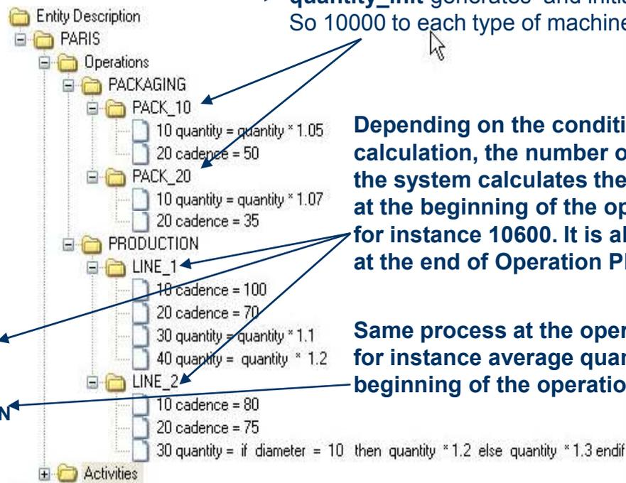
`quantity_init` generates and initializes the `quantity` variable; So 10000 to each type of machine
